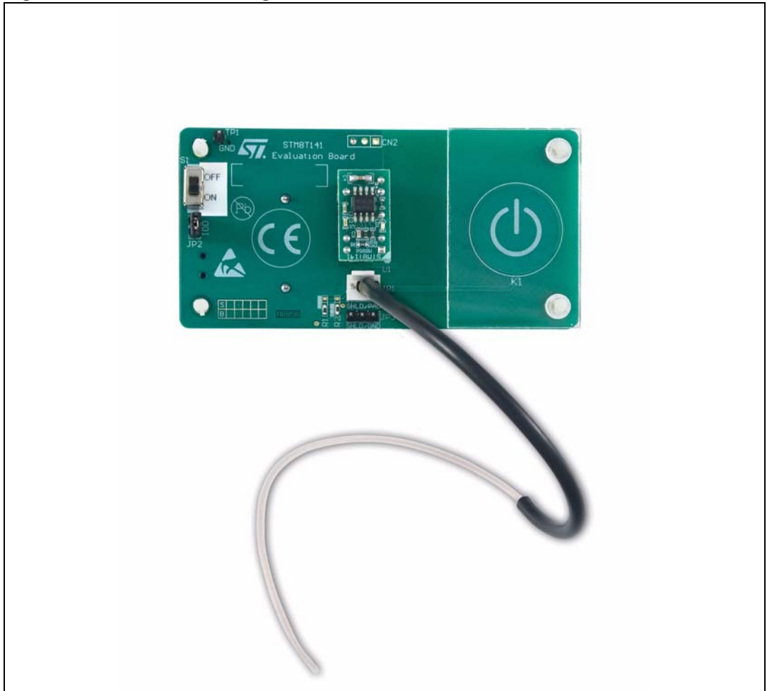
Figure 10. On-board sensing electrode with external antenna
