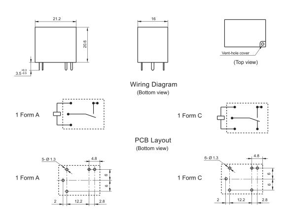
Remark: 1) In case of no tolerance shown in outline dimension: outline dimension  $\leq$ 1mm, tolerance should be  $\pm$ 0.2mm; outline dimension >1mm and  $\leq$ 5mm, tolerance should be  $\pm$ 0.3mm; outline dimension >5mm, tolerance should be  $\pm$ 0.4mm.
