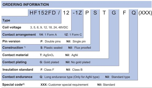
Notes: 1) Under the ambience with dangerous gas like H2S, SO<sub>2</sub> or NO<sub>2</sub>, plastic sealed type is recommended; Please test the relay in real applications.
