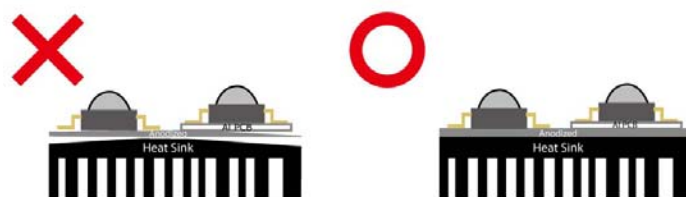
<Figure 31. Edixeon ® S series assemble with heat-sink>
