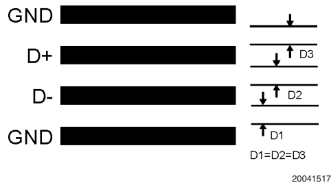
FIGURE 11. Ideal Diode Trace Layout
